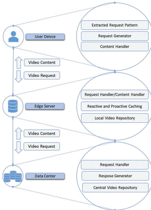
**Figure 1:** An overview of a proposed system with all basic components
