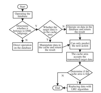
next action. The target data item is transmitted to the cache to determine whether the cache is full or not. If not, end the cache. If full, end the cache after replacing the data with the LRU algorithm.
