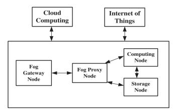
Figure 3: The internal hardware architecture of the fog layer
