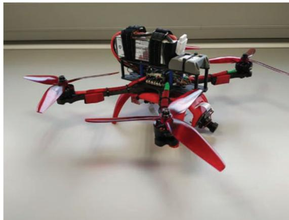
**Figure 7:** Assembled UAV-based security enabler
