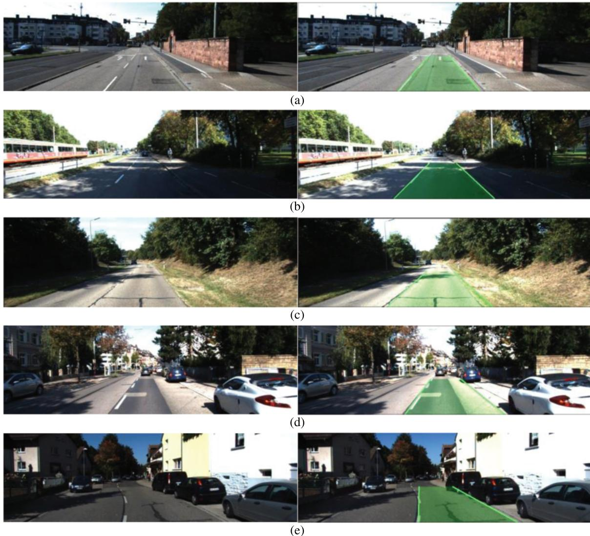
**Figure 9:** Original image frames of different challenges (left) and results of the proposed lane detection method (right)
