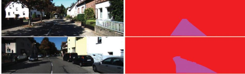
**Figure 5:** Examples of KITTI dataset images (left), and its lane's ground-truth (right)
