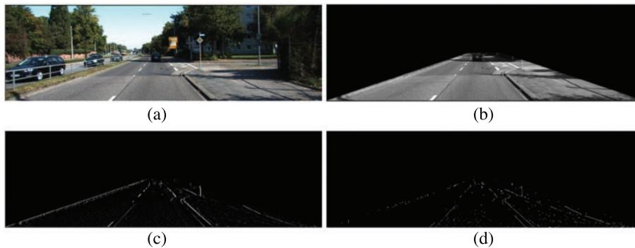
**Figure 2:** (a) Original image, (b) ROI, (c) vertical extracted edges, and (d) result of the preparation stage
