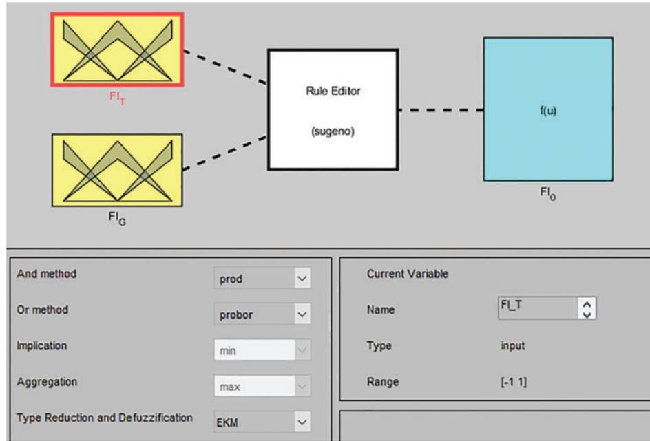
**Figure 5:** Main model editor of IT2 TSK with crisp interval inputs:  $(\widetilde{FI}_T)$ ,  $(\widetilde{FI}_G)$  and crisp output parameter:  $(\widetilde{FI}_O)$ , the optimized fire intensity value
