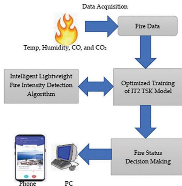
**Figure 3:** Proposed breakdown of the IT2 TSK fuzzy detection model with “fire status” decision making
