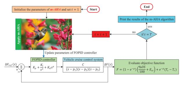
Figure 4: Block diagram detailing the implementation procedure of the proposed method to the cruise control system
