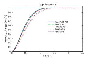
Figure 8: Velocity step responses for  $v_0 = 20 \ km/h$
