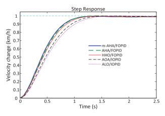
Figure 9: Velocity step responses for  $v_0 = 35 \ km/h$
