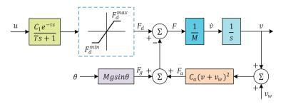
Figure 2: Cruise control system's dynamic model
