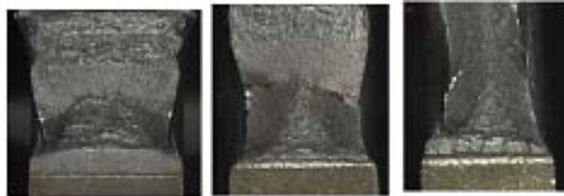
Figure 2: Fracture surface of three point bend specimen.
