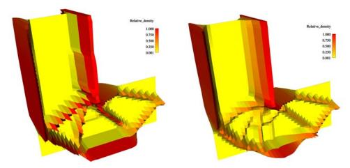
Figure 2: Local approach with q=1 (F=18.2%  $F_o$ ) (left) and global approach  $\mu=20$ , (F=17.6%  $F_o$ ) (right),  $\varepsilon=0.01$  and p=4, (Thickness multiplied by a factor of 0.5) and Bendsøe [8].
