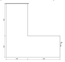
Figure 1: L-shape beam (units in meters).
