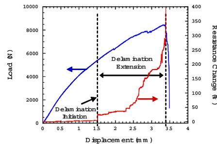
Figure 4: Load/displacement and resistance response of a 5-ply unidirectional composite with the center ply cut to initiate delamination.
