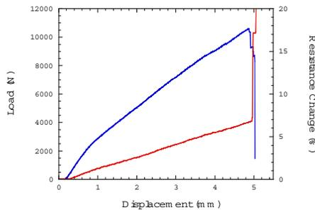
Figure 3: Load/displacement and resistance response of a unidirectional composite.
