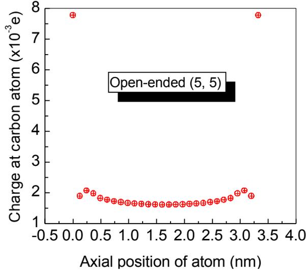
Figure 1: Charge distribution of a single walled nanotube in an infinite electric field.
