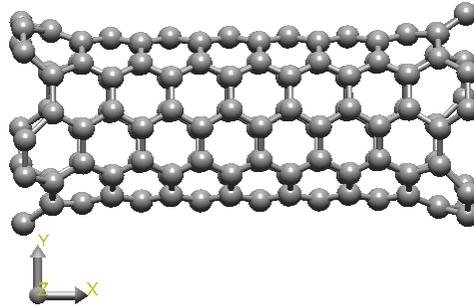
Figure 2: Electric-charge-deformed armchair (5, 5) carbon nanotube.
