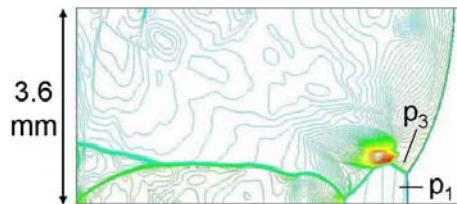
Figure 2: Instantaneous pressure contours of the detonation front ( p_1 , post-incident shock pressure; p_3 , post-reflected shock pressure).
