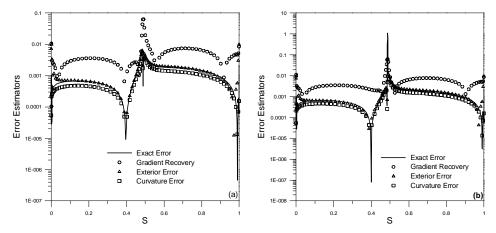
Figure 2: Joukowski airfoil cambered, panel number, for n = 300 linear panels, and for two different attack angles: (a)  $\alpha = 0^{\circ}$  and (b)  $\alpha = 3^{\circ}$ .
