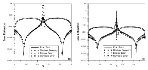
Figure 1: Joukowski airfoil without camber, for n = 300 linear panels, and for two different attack angles: (a)  $\alpha = 0^{\circ}$  and (b)  $\alpha = 3^{\circ}$ .
