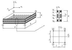
Figure 4: The rectangular Hybrid Assumed-Strain Laminated element (HASL).
