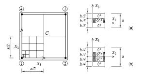
Figure 11: Simply-supported square laminated plate under distributed loads: the pattern of mesh refinement is partially shown. In (*a*) the [0/90/0] three-layer laminate is shown, in (*b*) the [0/90/90/0] four-layer one.
