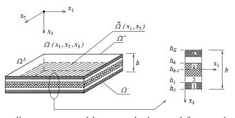
Figure 1: Coordinate system and layer numbering used for a typical laminated plate.
