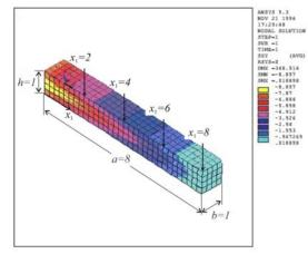
Figure 9: Distribution of shear stress  $\sigma_{13}$  for the [0/90/90/0] laminated plate (with a/h = 1) subjected to uniformly distributed load, analyzed with ANSYS brick elements: the finite element mesh is also shown.
