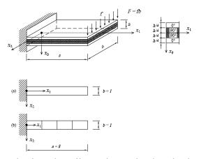
Figure 5: Four-layer laminated cantilever plate under shear load at the free end. (*a*) One element discretization; (*b*) Four elements discretization.
