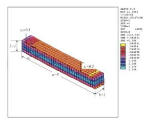
Figure 6: Distribution of shear stress  $\sigma_{13}$  for the [0/90/90/0] laminated plate (with a/h = 1) subjected to tip line-load, analyzed with brick elements: the finite element mesh is also shown.
