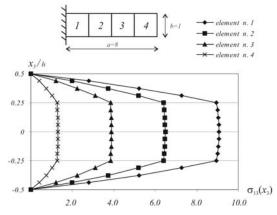
Figure 10: Distribution of shear stress  $\sigma_{13}$  along the thickness for the [0/90/90/0] laminated plate (a/h = 1) under uniformly distributed load: comparison between HASL and brick model results.
