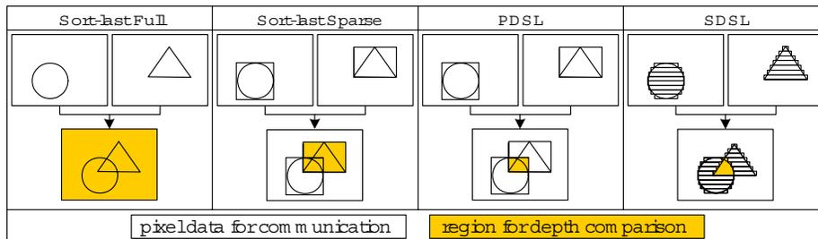
Figure 2: Pixel data for communication and depth comparison in sorting algorithms
