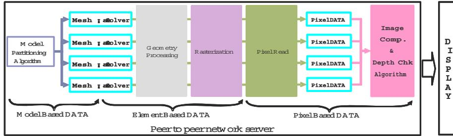
Figure 1: Parallel rendering system dedicated to distributed parallel finite element analysis
