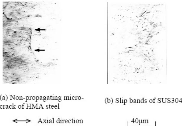
Figure 3: Specimen's surface state subjected to the stress amplitude of fatigue limit by  $1 \times 10^7$  cycles
