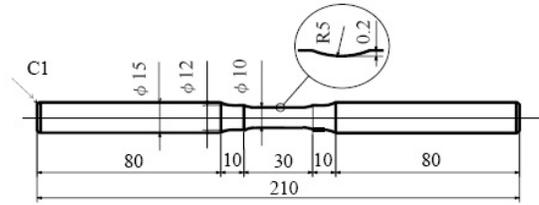
Figure 1: Shape and dimensions of specimen
