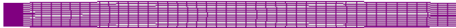
Figure 8: Refined mesh with mesh quality improvement: Max. aspect ratio 5.3 and average aspect ratio 4.6
