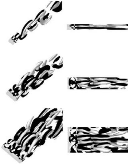
Figure 4: B-mode vortex shedding: comparison of streamwise components of vortexes for  $\pi d/2$ (top),  $\pi d$ (middle),  $2\pi d$ (bottom) at  $Re=1000$
