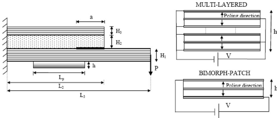
Figure 1: Drop-ply configuration and piezoelectric patch configurations.
