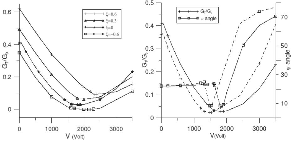
Figure 2: ERR distr. (left);  $G_T/G_0$  and  $\Psi$  for  $\xi=0$  (right: solid adhesive, dashed perfect).
