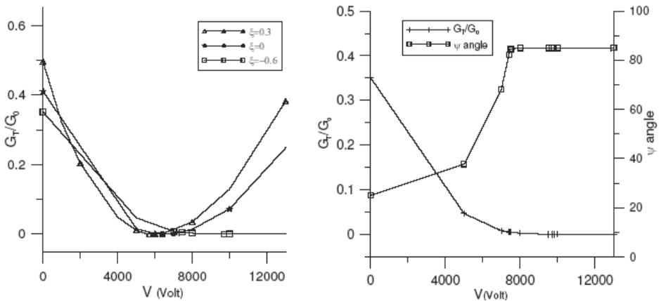
Figure 3: ERR distr. (left);  $G_T/G_0$  and  $\Psi$  for  $\xi = -0.6$  (right).
