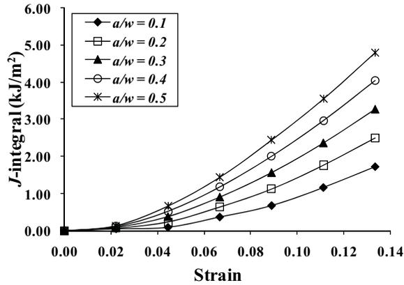
Figure 2:  $J$ -integral experimental data versus strain at various  $a/w$ .
