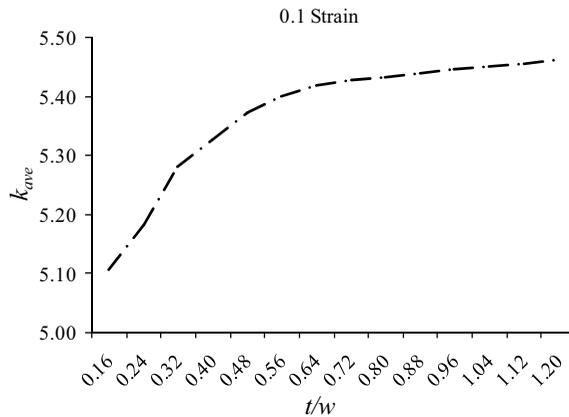
Figure 6:  $k_{ave}$  versus thickness and width ratio at  $a/w = 0.5$  and 10 percent strain.
