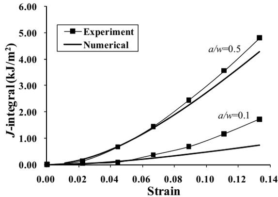
Figure 3:  $J$ -integral values from the experiment compare with those from the numerical for different crack length per width ratio ( $a/w$ ).
