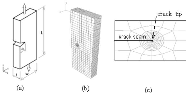
Figure 1: (a) specimen dimensions, (b) model meshing, (c) crack tip.
