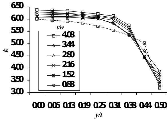
Figure 4:  $k$  along the thickness for different  $t/w$  at  $a/w = 0.5$  and 10 percent strain.
