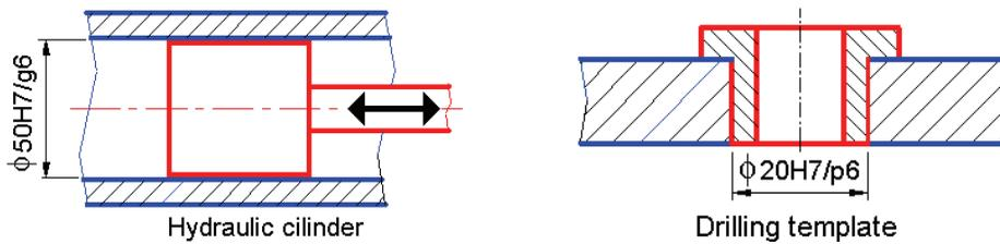
Figure 1: (a) Radial clearance fit. (b) Radial interference fit.
