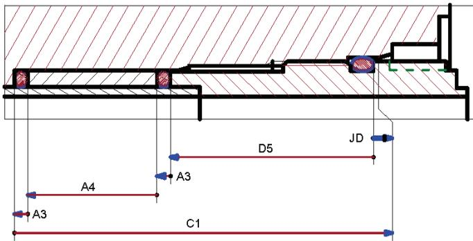
Figure 7: Dimensional chain for the functional condition JD.
