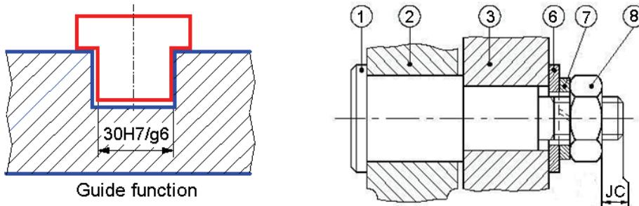
Figure 2: (a) Longitudinal clearance fit. (b) Functional condition JC.
