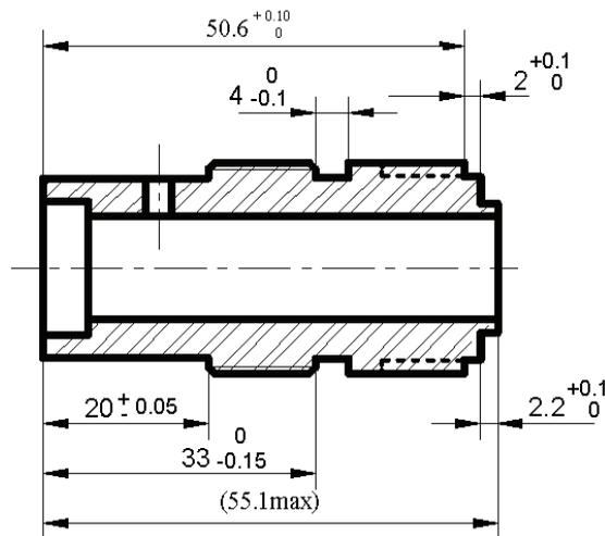
Figure 8: Functional dimensions for part # 5.
