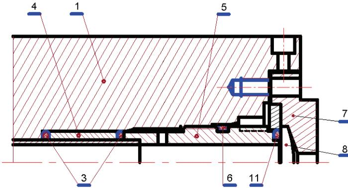
Figure 5: Front head of a CO2 laser beam prototype.
