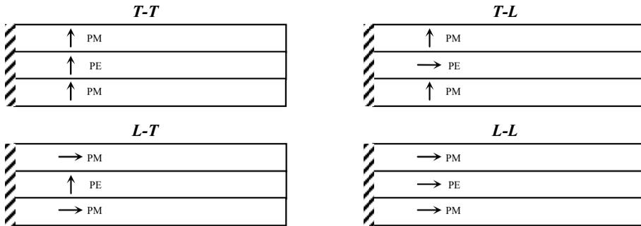
Figure 1: Tri-layered magnetoelectric composite working modes arrangements
