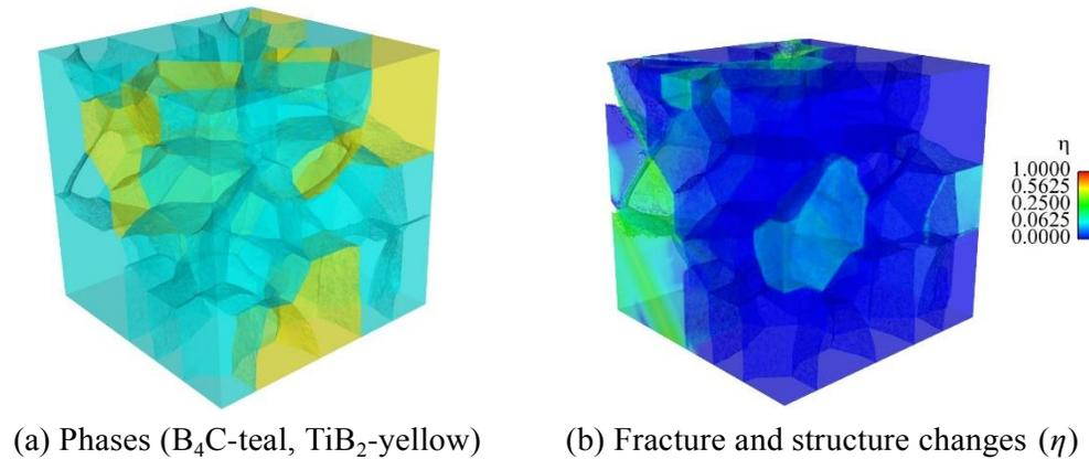
**Figure 1:** Microstructure rendering (FE mesh) and  $\eta$  contours for B<sub>4</sub>C-TiB<sub>2</sub> at compressive strain of 0.7% with fractured elements ( $\xi > 0.8$ ) visually removed
