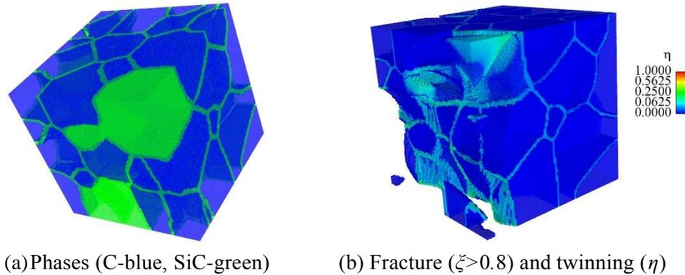
**Figure 2:** Microstructure and  $\eta$  contours for diamond-SiC at 0.6% strain
