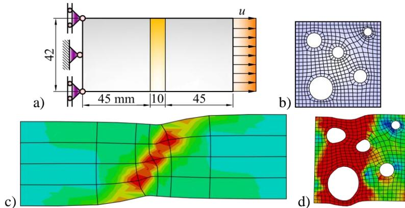
**Figure 2:** a) Geometry and loading of strip, b) heterogeneous RVE, c) damage response of macromodel, d) damaged microstructural volume element
