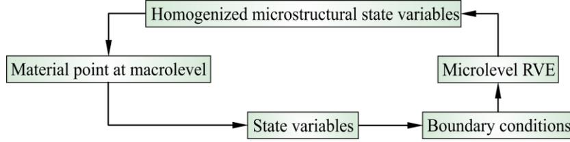
**Figure 1:** Two-scale computational scheme
