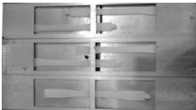
Figure 2. Specimens placed for ageing in QUV weatherometer
