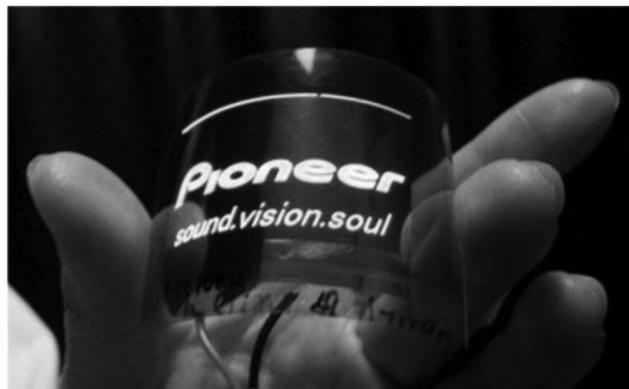
**Figure 7** Flexible display on CNF substrate. (Reprinted with permission from [56]; Copyright 2009 Elsevier)
