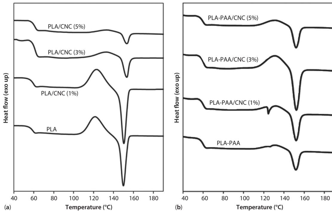
**Figure 2** Second run DSC scan curves of PLA (a) and PLA-g-PAA (b) loaded with cellulose nanocrystals. The plots are offset for clarity.
