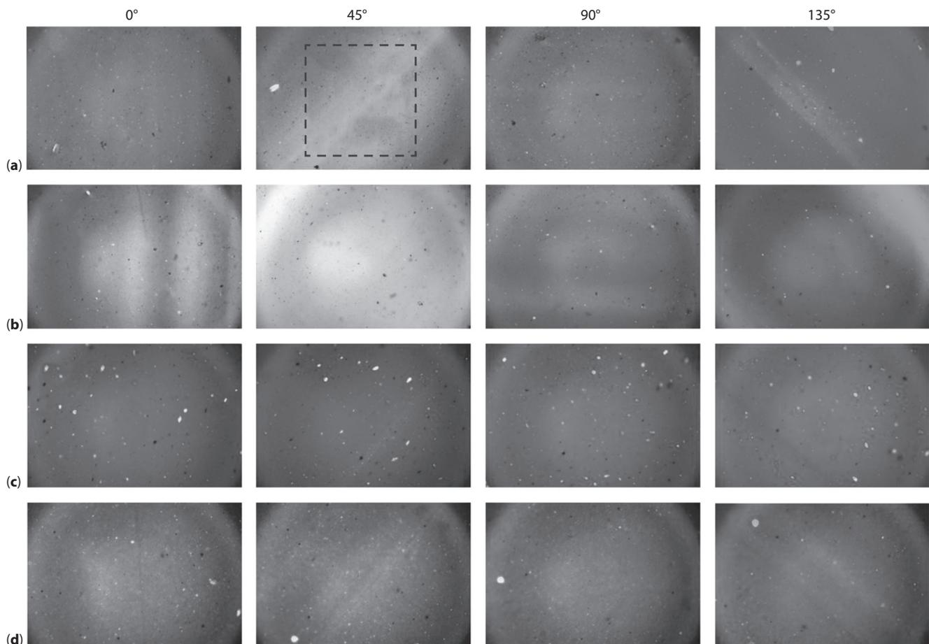
**Figure 4** Polarized-light microscopy PLA (a, b) and PLA-g-PAA/CNC nanocomposites (c, d) using a first order red filter. (a, c) 1% and (b, d) 3% CNC nanocomposites. The dotted square in the picture represents the size of the area used for the color quantification. Length of each image: 1.5 mm.
