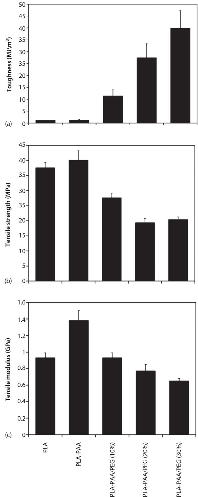
**Figure 5** Mechanical properties of PLA-g-PAA/PEG blends: (a) toughness, (b) tensile strength, and (c) tensile modulus.
