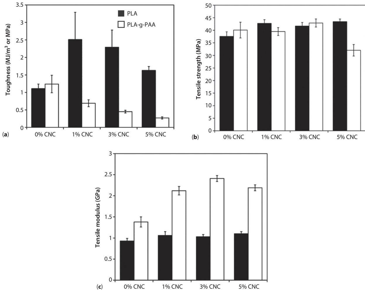
**Figure 1** Mechanical properties of PLA (■) and PLA-g-PAA/CNC (□) nanocomposites: (a) toughness, (b) tensile strength, and (c) tensile modulus.
