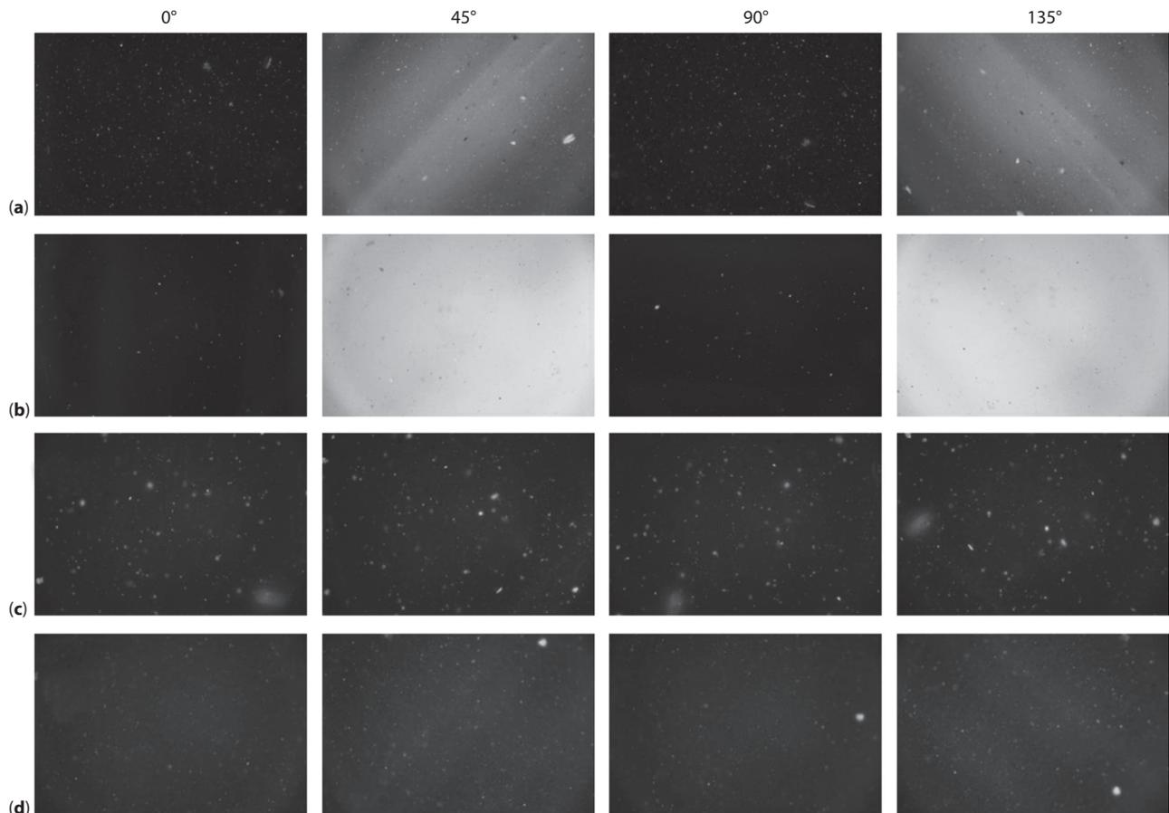
**Figure 3** Polarized-light microscopy of PLA (a, b) and PLA-g-PAA/CNC nanocomposites (c, d). (a, c) 1% and (b, d) 3% CNC. Length of each image: 1.5 mm.
