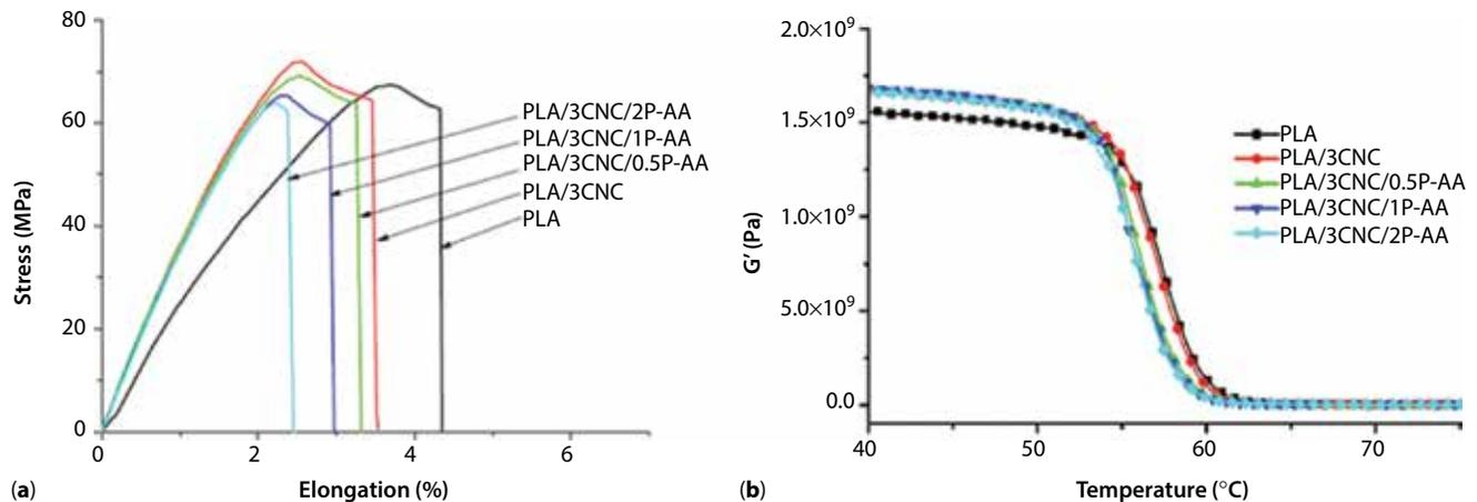
**Figure 5** Tensile stress-strain curves of (a) PLA and PLA/CNC/P-AA nanocomposites and (b) storage modulus as a function of temperature for PLA and PLA/CNC/P-AA nanocomposites.
