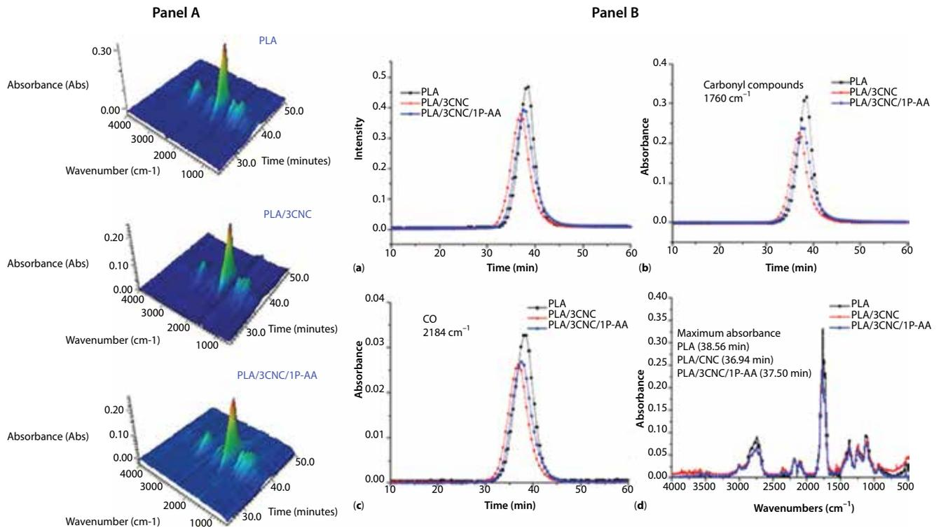
**Figure 2** (Panel A) 3D TG-FTIR spectrum of gas phase in the thermal degradation of neat PLA, PLA/3CNC, PLA/3CNC/1P-AA. (Panel B) Absorbance of pyrolysis products for PLA, PLA/3CNC and PLA/3CNC/1P-AA vs time: (a) Total, (b) Carbonyl compounds, (c) CO, and (d) Maximum absorbance.
