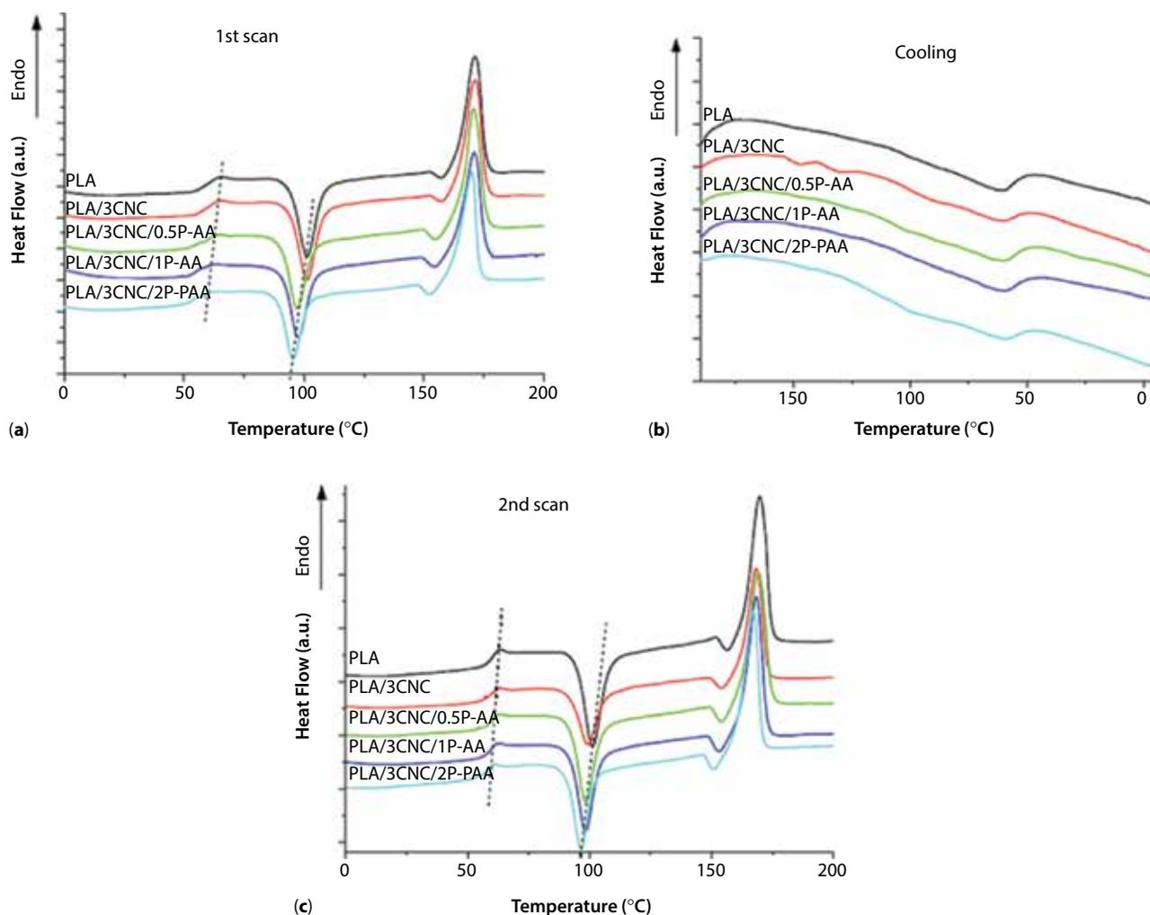
**Figure 3** DSC thermograms of PLA and PLA/CNC/P-AA nanocomposites during (a) 1<sup>st</sup> heating scan, (b) cooling and (c) 2<sup>nd</sup> heating scan.
