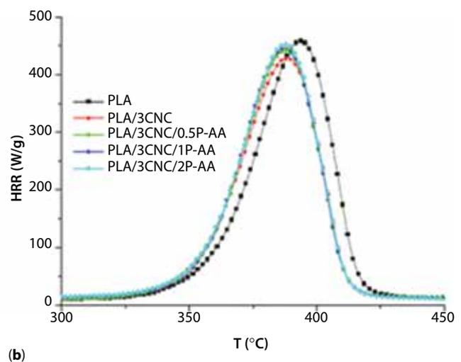
**Figure 1** HRR curves of (a) P-AA and (b) PLA and different PLA nanocomposite systems containing both CNC and P-AA, obtained by microcalorimeter tests.
