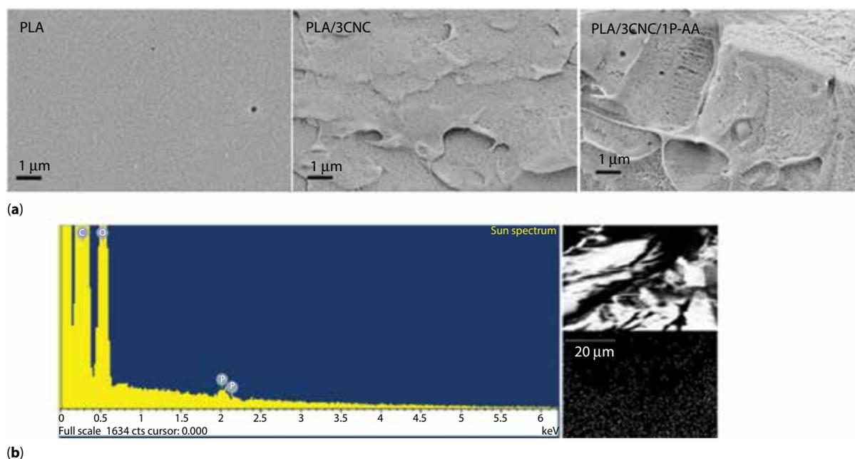
**Figure 6** (a) FESEM images of cryofractured cross sections for neat PLA, PLA/3CNC and PLA/3CNC/1P-AA systems. (b) EDX spectrum and phosphorus elemental distribution from SEM/EDS mapping for PLA/3CNC/2P-AA.
