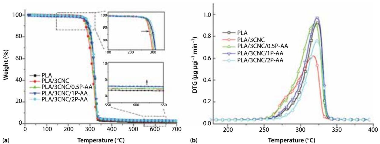
**Figure 4** (a) TG and (b) DTG curves of neat PLA and its nanocomposites containing both CNC and P-AA.
