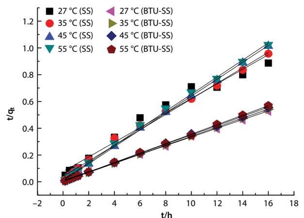
**Figure 8** The fitting of pseudo-second-order for adsorption of Ag(I) onto SS and BTU-SS at different temperatures.
