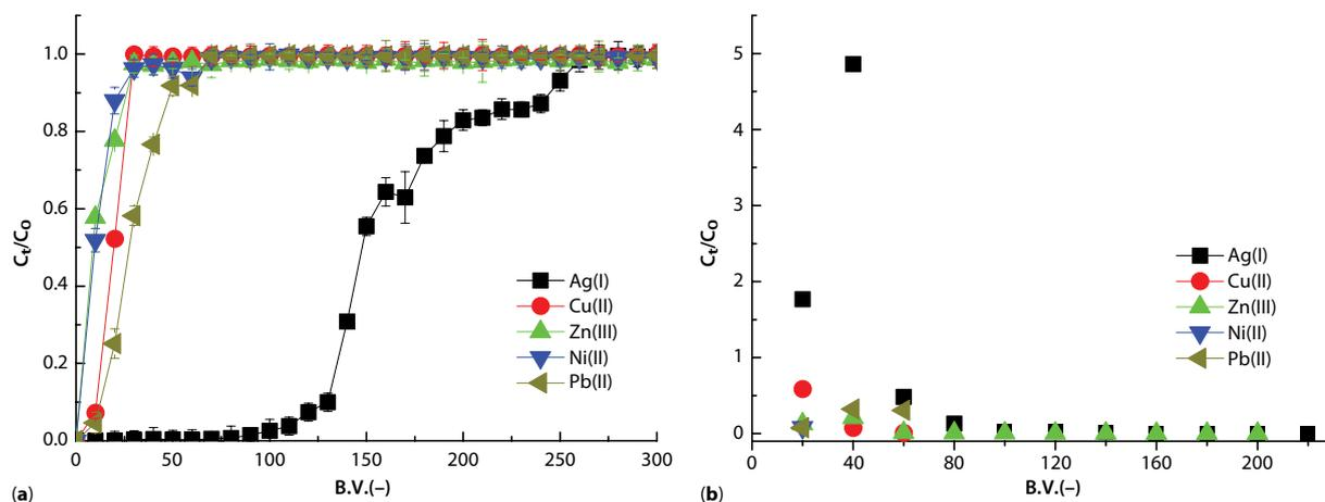
**Figure 11** Breakthrough curves (a) and elution curves (b) of metallic ions on BTU-SS in Ag(I)-Cu(II)-Zn(II)-Ni(II)-Pb(II) system. (Feed concentrations of metallic ions ( $\text{mg}\cdot\text{L}^{-1}$ ): Cu(II) = 602.3; Ni(II) = 534.8; Pb(II) = 398.7; Zn(II) = 53.8; Ag(I) = 113.6 with flow rate  $5.0\text{ cm}^3\cdot\text{h}^{-1}$ ; Eluent = 1.0 M thiourea in 1.0 M  $\text{HNO}_3$  with elution rate  $10.0\text{ cm}^3\cdot\text{h}^{-1}$ .)
