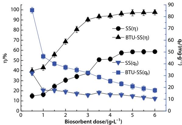
**Figure 4** Effect of biosorbent dose on adsorption of Ag(I); (pH = 5.0, t = 15 h, C<sub>0</sub>(Ag(I)) = 108.0 mg·L<sup>-1</sup>).
