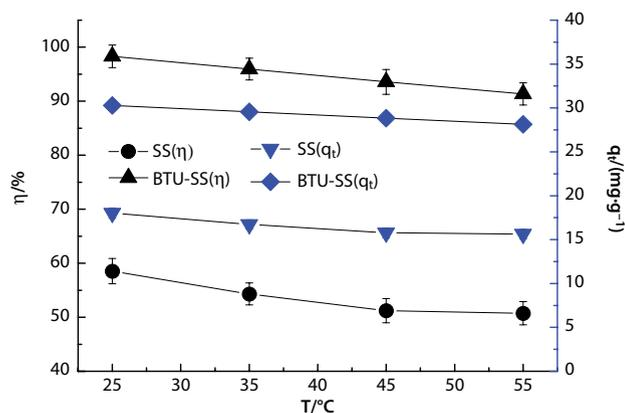
**Figure 6** Effect of temperature on adsorption of Ag(I); ( $t = 15$  h, pH = 5.0, biosorbent dose =  $3.5 \text{ g}\cdot\text{L}^{-1}$ ,  $C_0(\text{Ag(I)}) = 108.0 \text{ mg}\cdot\text{L}^{-1}$ ).
