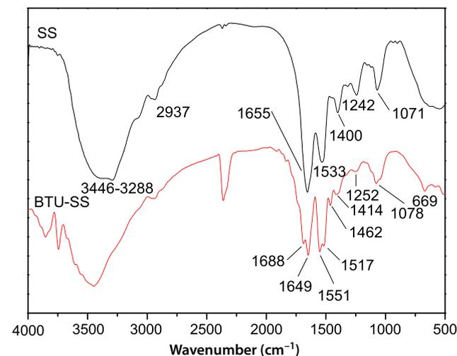
Figure 1 FTIR spectra of SS and BTU-SS.
