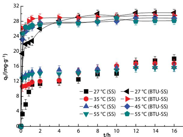
**Figure 7** Adsorption kinetics of SS and BTU-SS towards Ag(I) at different temperatures; (pH = 5.0, biosorbent dose = 3.5 g·L<sup>-1</sup>, C<sub>0</sub>(Ag(I)) = 108.0 mg·L<sup>-1</sup>).
