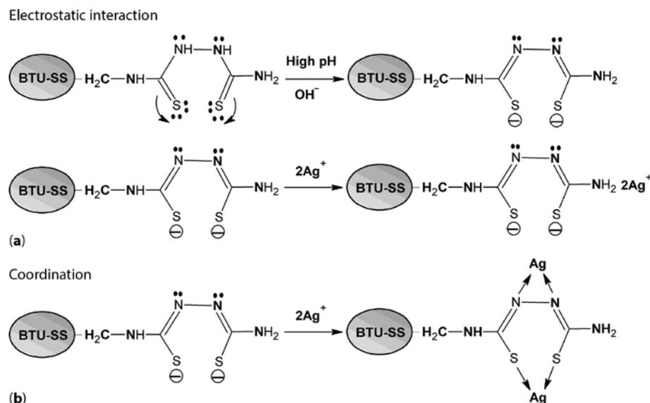
**Scheme 2** Presumable mechanism of adsorption of Ag(I) on BTU-SS.
