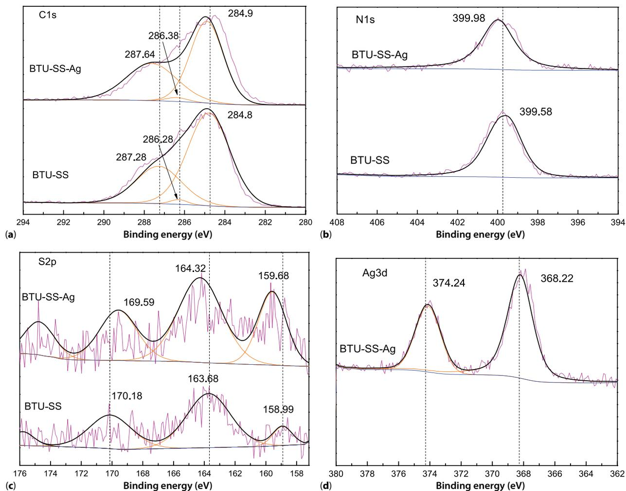
**Figure 14** X-ray photoelectron spectra of fresh and Ag(I)-loaded BTU-SS: (a) C1s, (b) N1s, (c) S2p and (d) Ag3d. The observed signals with noise are shown with non-smooth curves and the fitted lines with smooth curves in all spectra.
