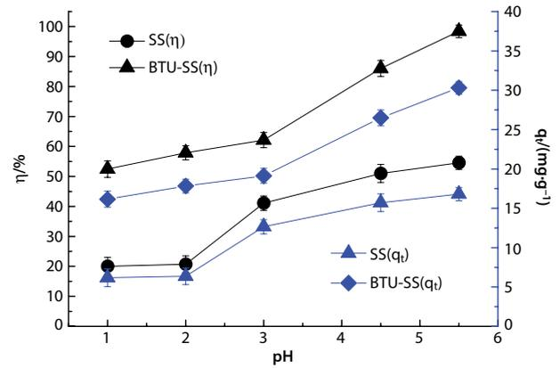
**Figure 5** Effect of pH on adsorption of Ag(I); (t = 15 h, biosorbent dose = 3.5g·L<sup>-1</sup>, C<sub>0</sub>(Ag(I)) = 108.0 mg·L<sup>-1</sup>).
