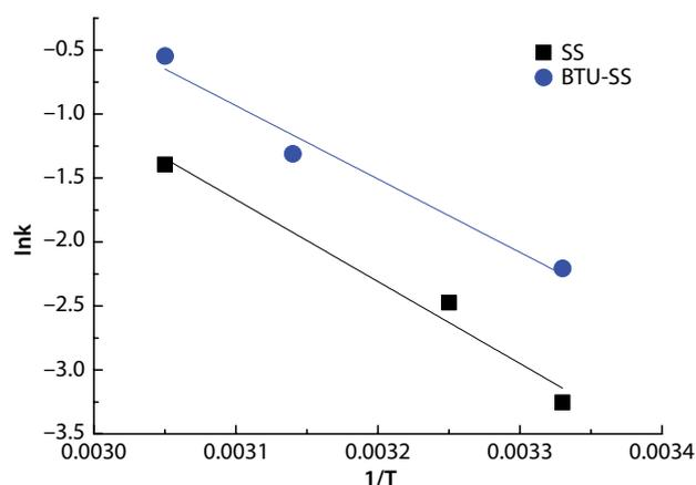
**Figure 9** Relationship between  $1/T$  and  $\ln k$  for adsorption of Ag(I) onto SS and BTU-SS.
