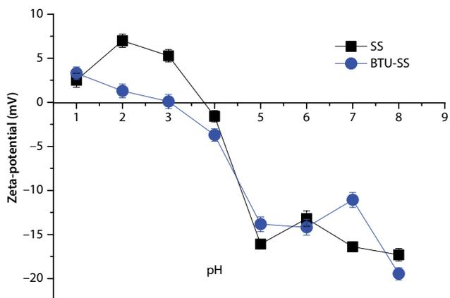
Figure 2 Zeta potential of SS and BTU-SS at different pH.
