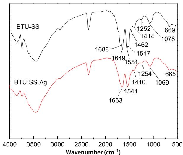
**Figure 13** FTIR spectra of fresh and Ag(I)-loaded BTU-SS.
