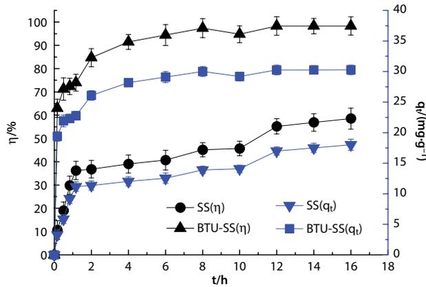
**Figure 3** Effect of contact time on adsorption of Ag(I); (pH = 5.0, biosorbent dose = 3.5 g·L<sup>-1</sup>, C<sub>0</sub>(Ag(I)) = 108.0 mg·L<sup>-1</sup>).
