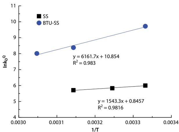
Figure 10 Van 't Hoff relationship between  $1/T$  and  $\ln K_D^\circ$  for adsorption of Ag(I) onto SS and BTU-SS.
