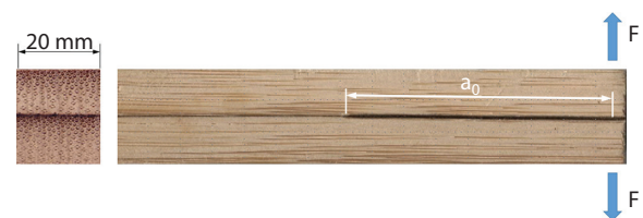
Figure 1 Double cantilever beam test specimen.
