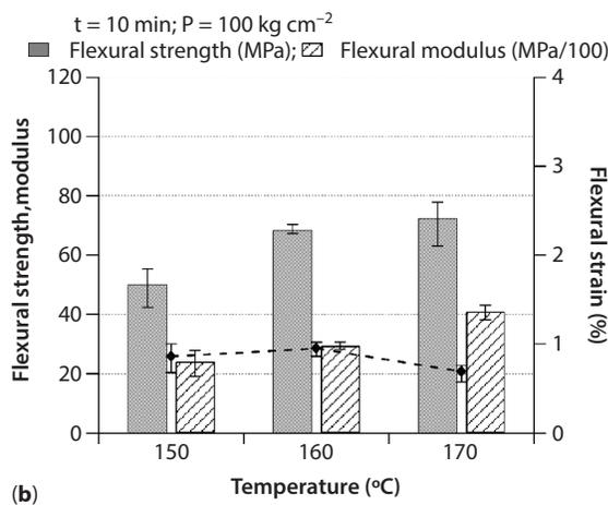
**Figure 2** Effects of processing temperature on (a) tensile and (b) flexural properties of banana fiber-reinforced composites.
