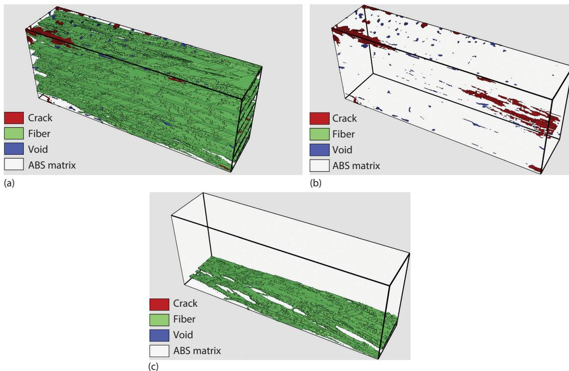
**Figure 9** A banana fiber-reinforced composite processed at 170 °C in 20 min and under 125 kg cm<sup>-2</sup>: (a) Three-dimensional whole structures, (b) void and crack distribution, and (c) 3D structure of one layer.
