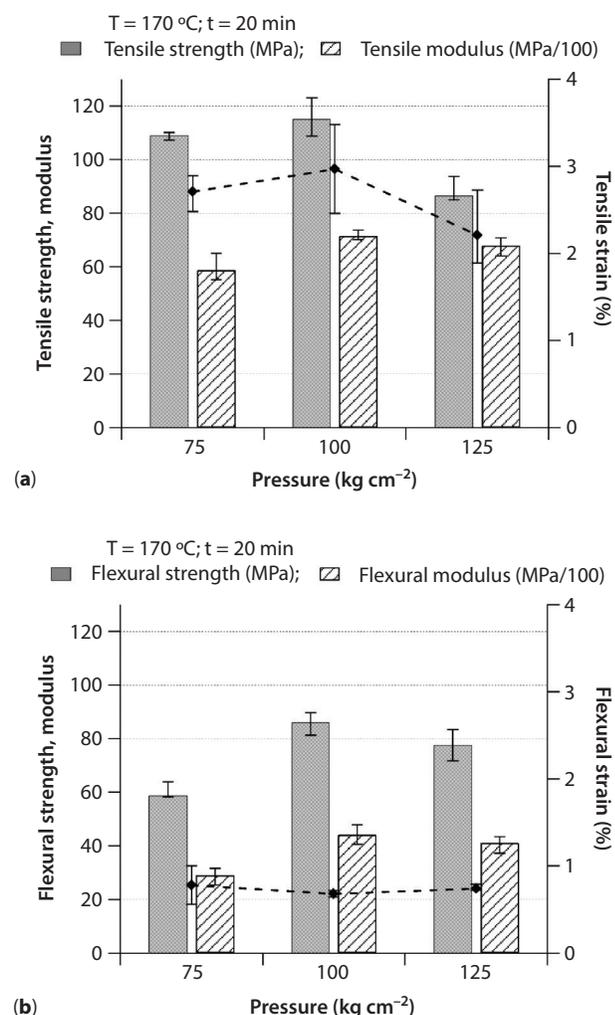
Figure 8 Effects of processing pressure on (a) tensile and (b) flexural properties of banana fiber-reinforced composites.
