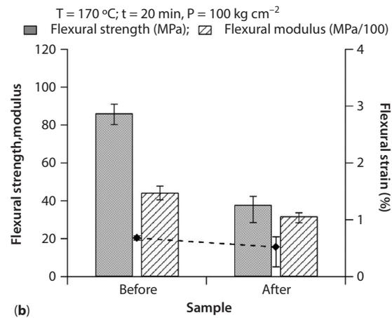
**Figure 14** (a) Tensile and (b) flexural properties of banana fiber-reinforced composites prepared at  $T = 170\text{ }^{\circ}\text{C}$ ,  $P = 100\text{ kg cm}^{-2}$  in 20 min before and after water absorption.
