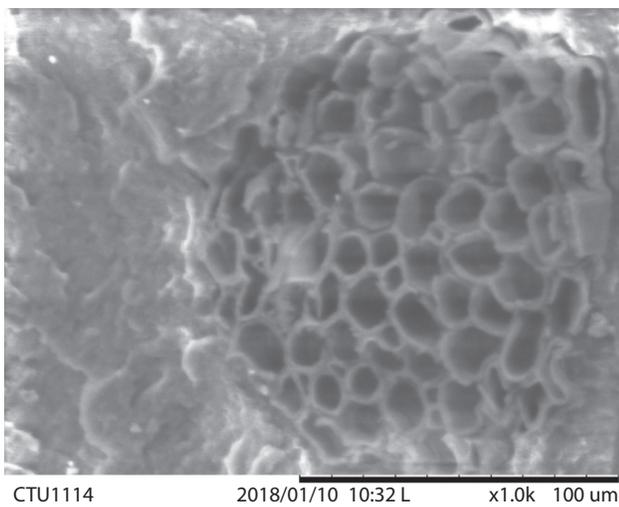
**Figure 13** Cross section of banana fiber-reinforced composite prepared at  $T = 170\text{ }^{\circ}\text{C}$ ,  $P = 100\text{ kg cm}^{-2}$  in 20 min after tensile test.
