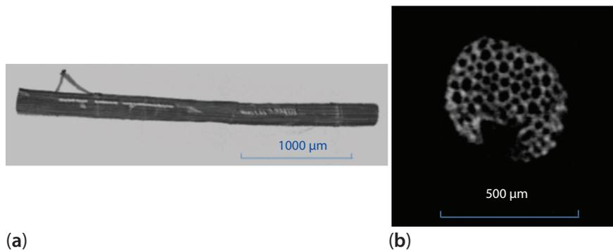
**Figure 1** Structure of banana fibers observed by X-ray CT (a) along the length and (b) at cross section of the fibers.
