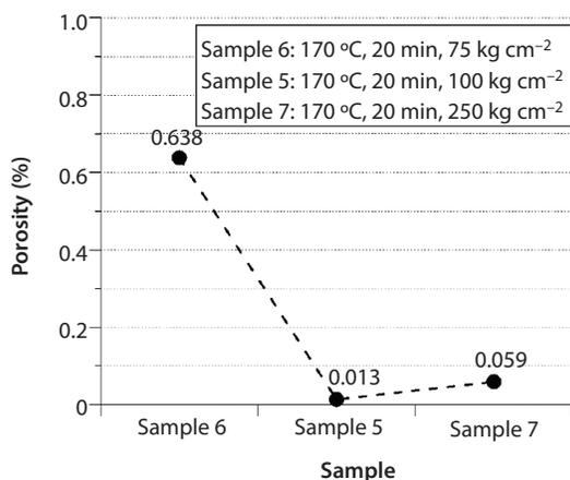
**Figure 10** Porosity in banana fiber-reinforced composites processed under various pressures.
