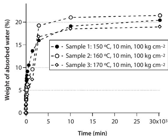
**Figure 4** Water absorption of banana fiber-reinforced composites processed at various temperatures.
