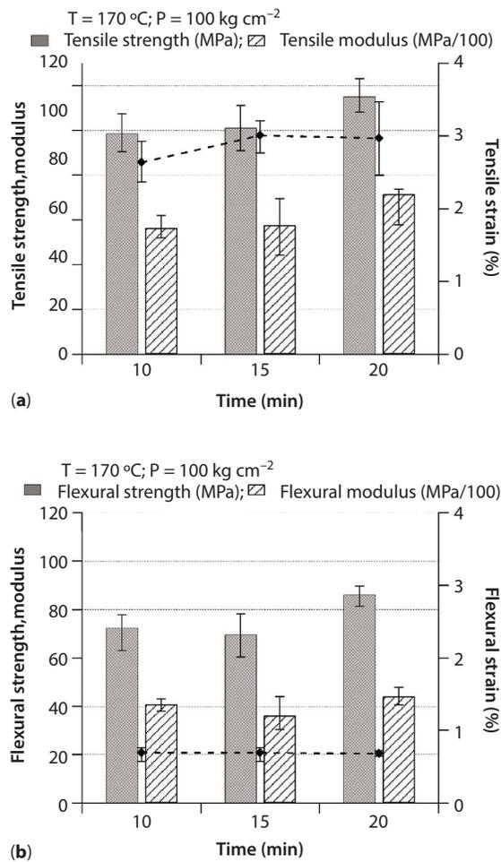
**Figure 5** Effects of processing time on (a) tensile and (b) flexural properties of banana fiber-reinforced composites.
