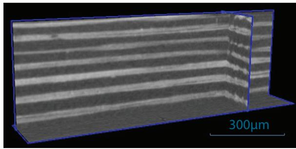
**Figure 12** 3D model reconstruction of a banana fiber-reinforced composite prepared at  $T = 170\text{ }^{\circ}\text{C}$ ,  $P = 100\text{ kg cm}^{-2}$  in 20 min.
