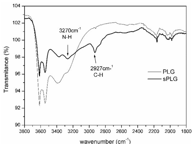
**Figure 1:** FTIR spectra of PLG and sPLG nanofillers
