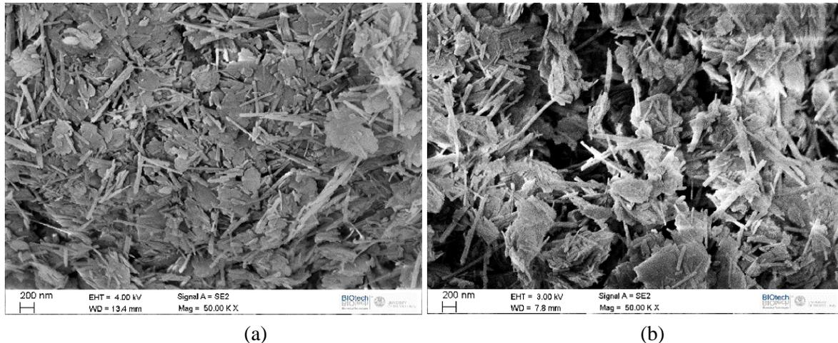
**Figure 3:** SEM images of the (a) PLG and (b) sPLG nanofillers
