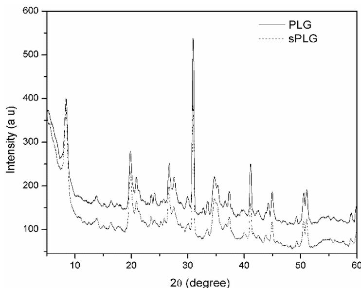
**Figure 2:** X-Ray diffraction patterns of PLG and sPLG nanofillers
