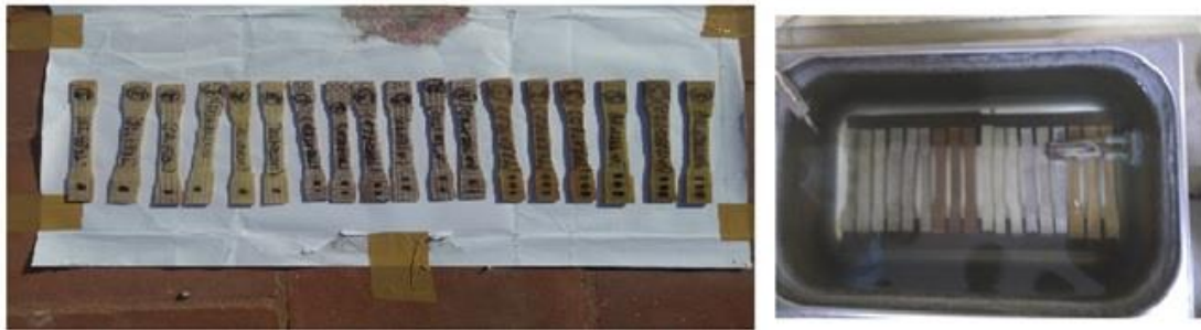
Figure 9: Tensile Test specimens in Hygrothermal setup
