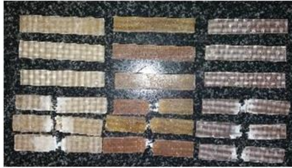
Figure 7: Impact test specimens
