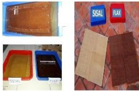
Figure 1: NaOH treatment of flax and sisal fiber
