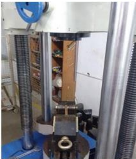
Figure 5: Flexural Test setup
