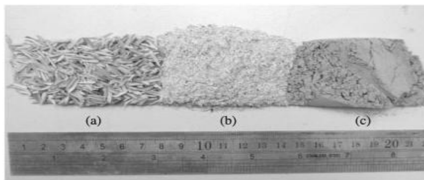
Figure 3: (a) Rice bran, (b) Rice Husk Ash (c) Rice Husk Ash ground
