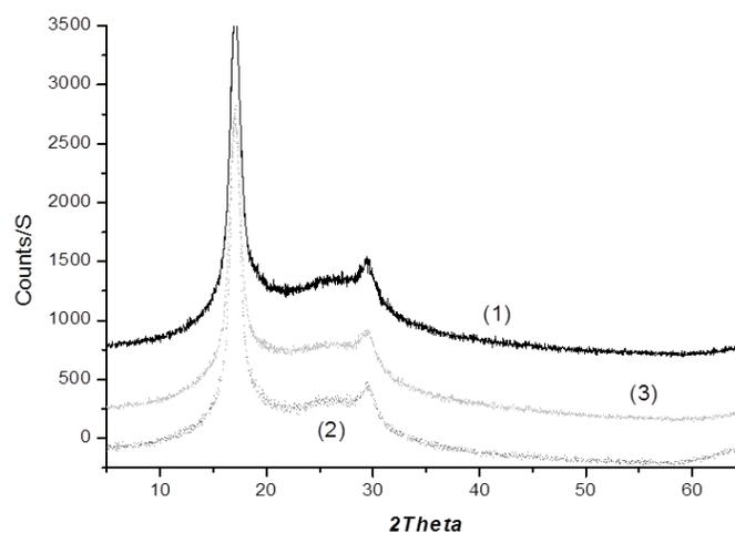
**Figure 4:** X-Ray Analysis of untreated acrylic (1), cationized acrylic by Croscolor DRT (2) and amidoximated (3) fabrics
