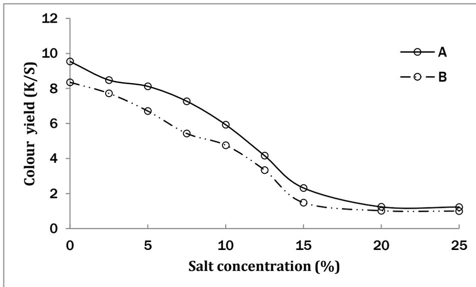
**Figure 9:** Effect of the salt concentration on the colour yield (K/S) for cationized (A) and amidoximated (B) acrylic fibers
