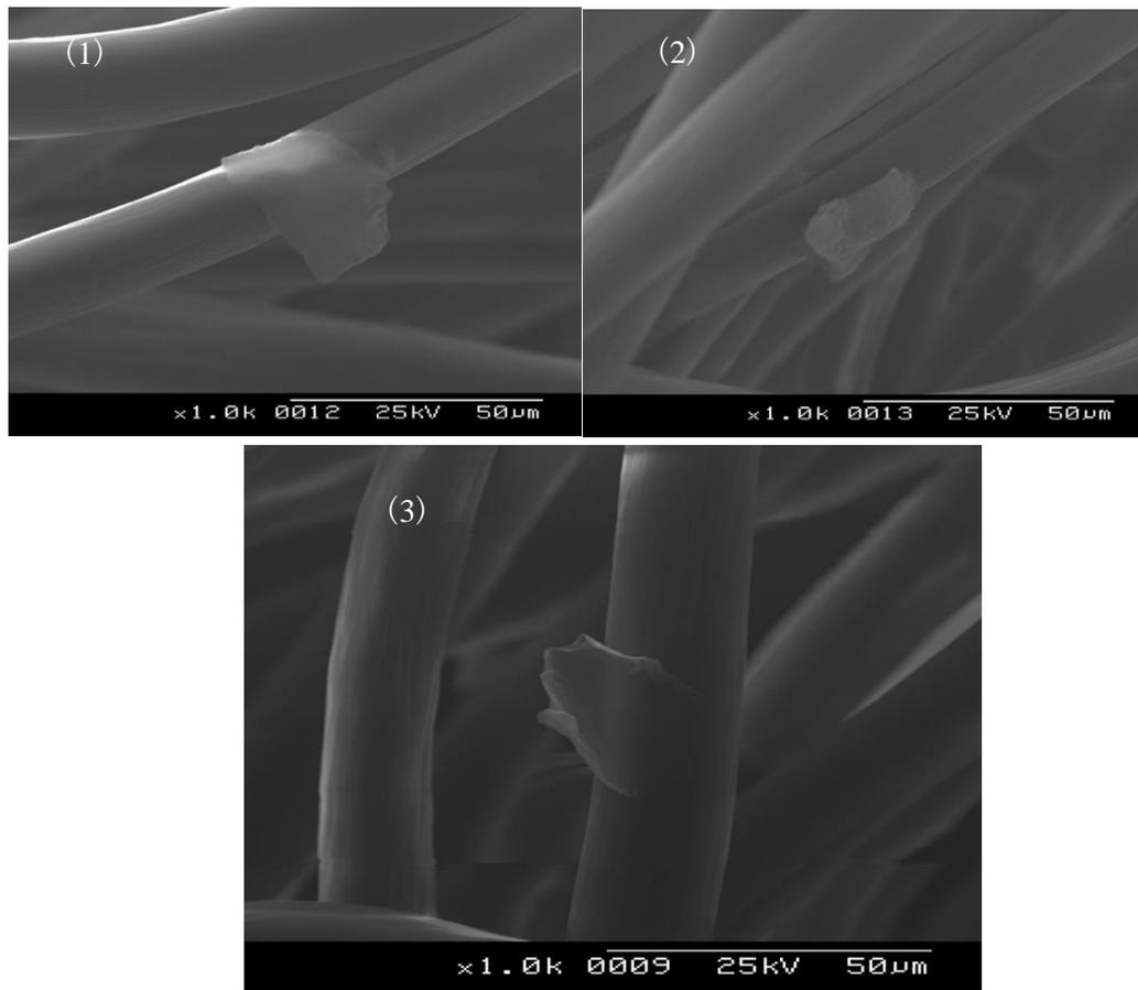
**Figure 5:** SEM photographs of untreated fibres (1), cationized acrylic fibres (2) and amidoximated acrylic fibres (3)
