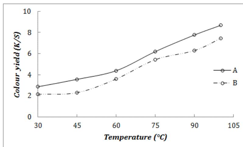
**Figure 7:** Effect of the dye bath temperature on the colour yield (K/S) for cationized (A) and amidoximated (B) acrylic fibers
