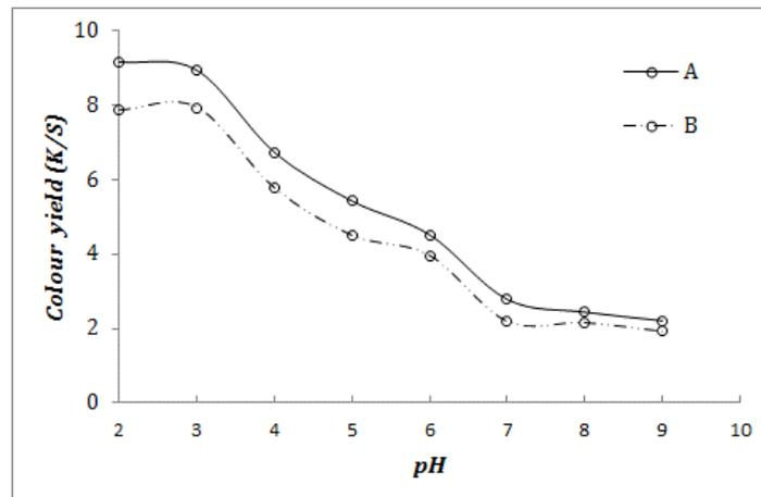
**Figure 6:** Effect of the dye bath pH on the colour yield (K/S) for cationized (A) and amidoximated (B) acrylic fibers
