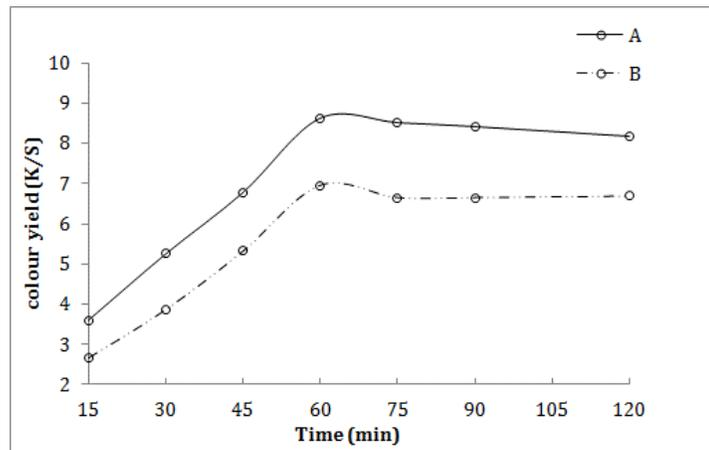
**Figure 8:** Effect of the dyeing time on the colour yield (K/S) for cationized (A) and amidoximated (B) acrylic fibers
