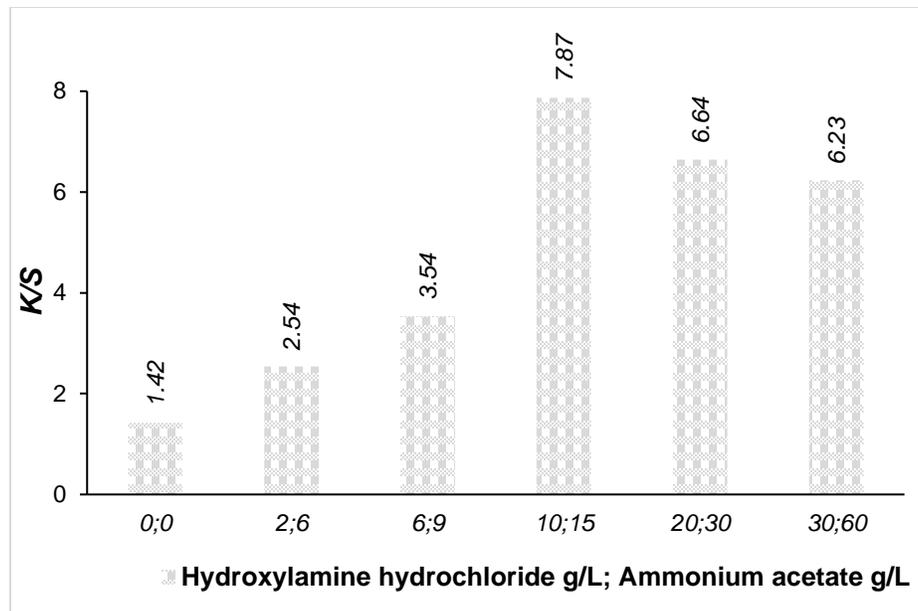
**Figure 3:** Effect of the hydroxylamine hydrochloride and ammonium acetate concentrations, on the colour yield (K/S) of dyed modified acrylic fabrics
