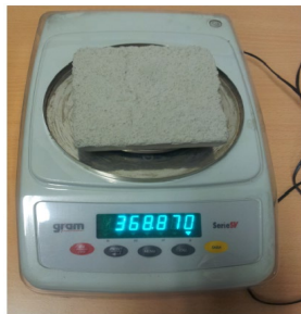
Figure 5: Sample of cement mortar without additive
