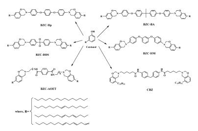
Figure 4: Some difunctional cardanol based benzoxazine resins
