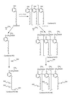
Figure 10: Synthesis of cardanol-based polyols by using thiol-ene reaction
