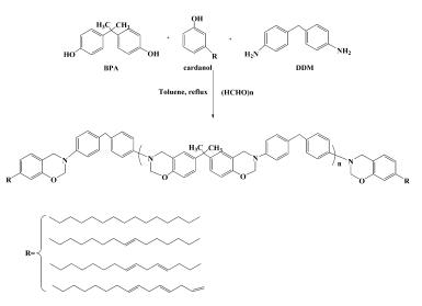
**Figure 6:** Synthesis of MCBO(BPA-ddm)C, MCBO(BPA-ddm)C-P and MCBO(BPA-ddm)P based on BPA, DDM, phenol and candanol
