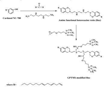
Figure 5: Synthesis reaction of Bnz and GPTMS-modified Bnz
