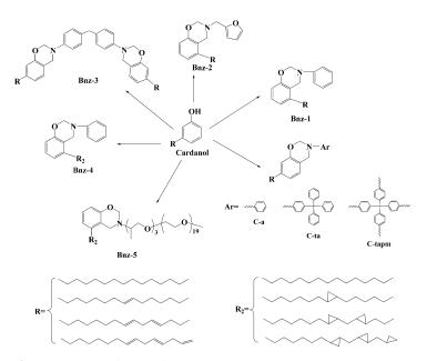
Figure 3: Structures of monofunctional Cardanol based benzoxazine resins
