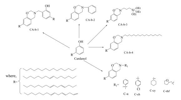
Figure 2: Some monofunctional Cardanol based benzoxazine resins
