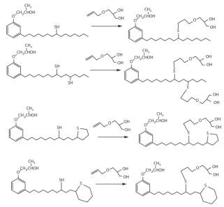
Figure 9: Synthesis of polyols from photochemical thiol-ene reactions of cardanol based derivatives
