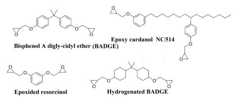
Figure 8: Chemical structure of epoxidized cardonal based curing agents
