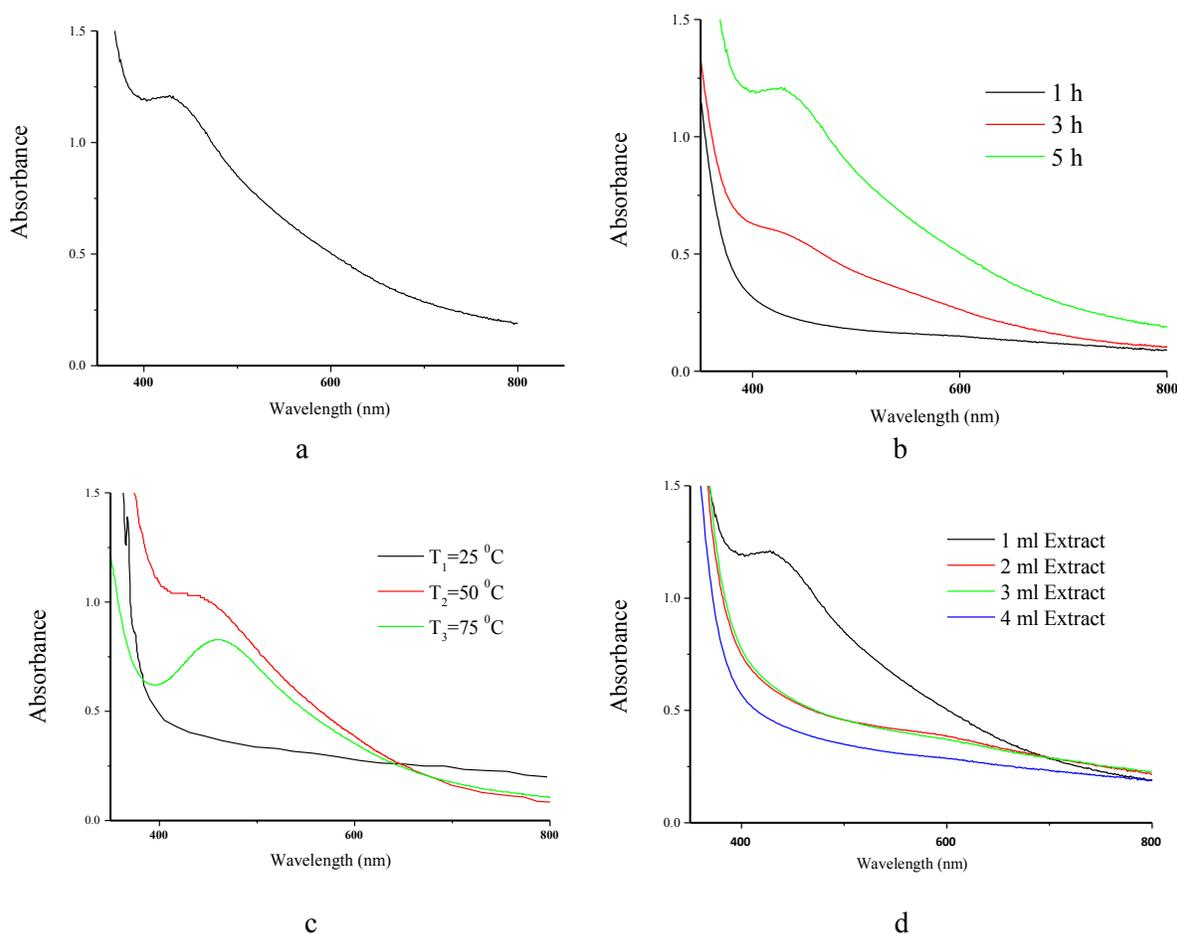
**Figure 4:** UV-Visible spectra of synthesized AgNPs at 437 (a), different procedure time ( $t_1 = 1$ ,  $t_2 = 3$ ,  $t_3 = 5$  hrs) (b), different reaction temperature ( $T_1 = 25^\circ\text{C}$ ,  $T_2 = 50^\circ\text{C}$ ,  $T_3 = 75^\circ\text{C}$ ) (c), and different concentrations of mullein extract (1, 2, 3, and 4 ml of 2.5 %w/w solution) (d)
