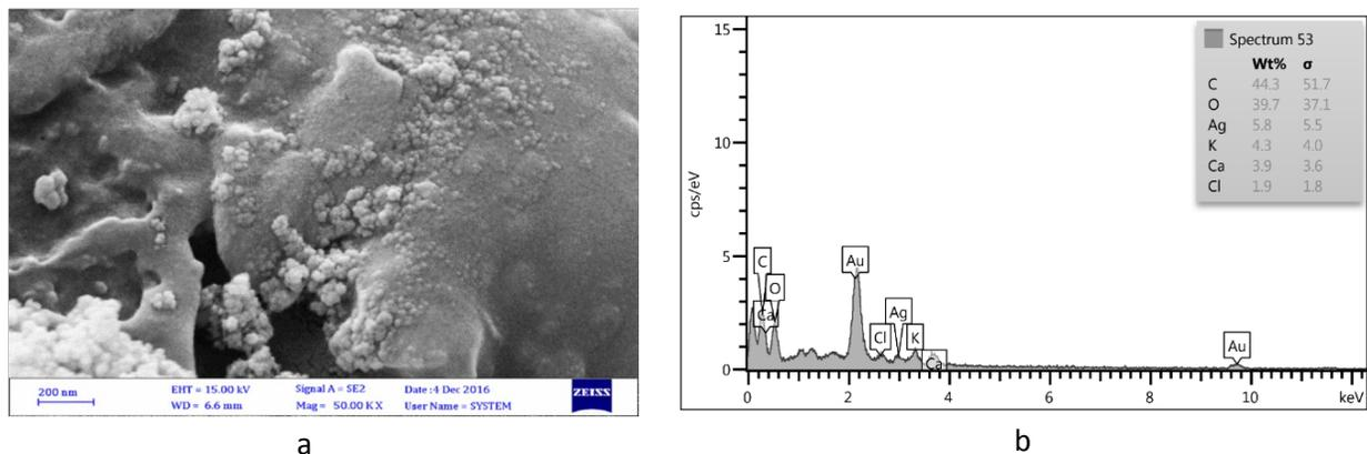
**Figure 1:** SEM image micrograph (a) and EDX profile of synthesized AgNPs (b)
