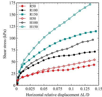
**Figure 3:** Experimental curves from the shear test on plant aggregates. R: rice husk-H: hemp shiv-50, 100 and 150 are normal stresses in kPa
