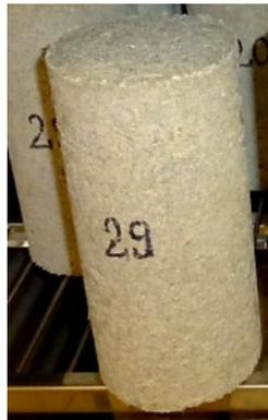
**Figure 6:** Specimen of a bio-aggregate-based concrete
