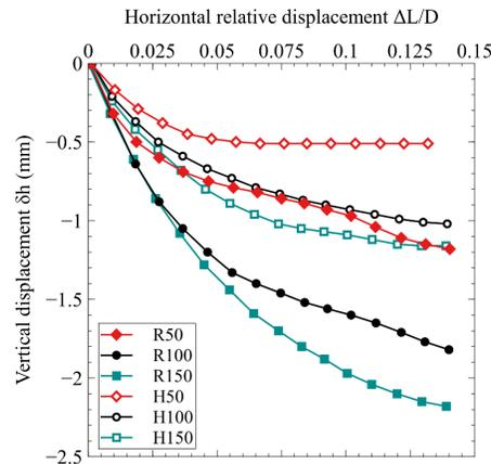
**Figure 4:** Vertical displacement versus horizontal relative displacement during the shearing stage. See Fig. 3 for the caption
