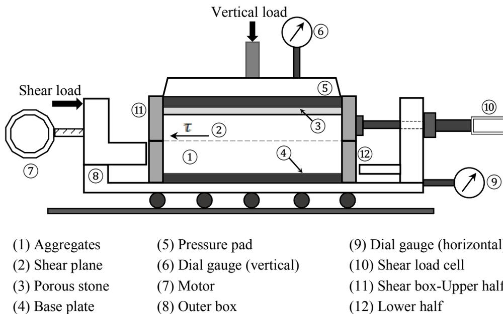
Figure 2: Shear box apparatus
