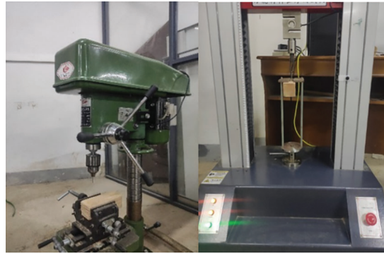
Figure 3: The test of nail holding strength
