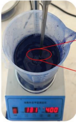
(a) Methylene blue adsorption test
