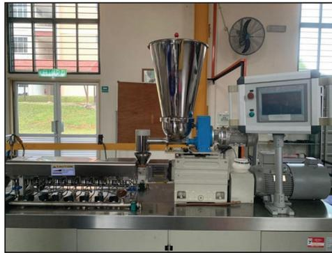
**Figure 5:** Twin screw extruder**Table 5:** Parameter filament extrusion
