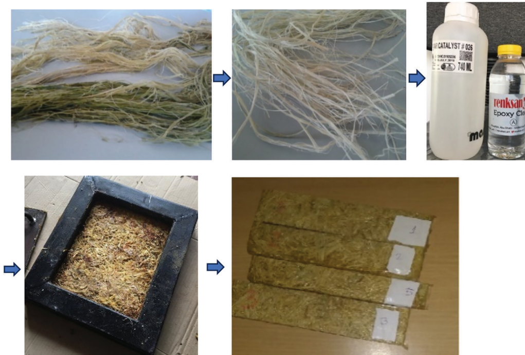
Figure 3: Preparation of Leptadenia pyrotechnica fiber-reinforced composite samples
