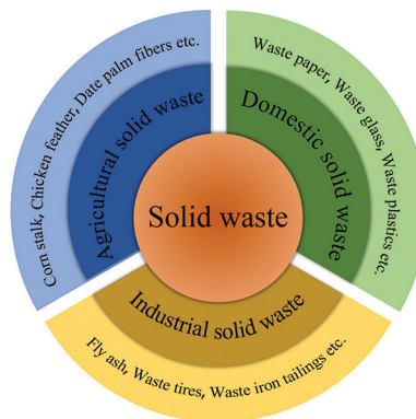
Figure 2: Schematic diagram of solid waste sources and classification
