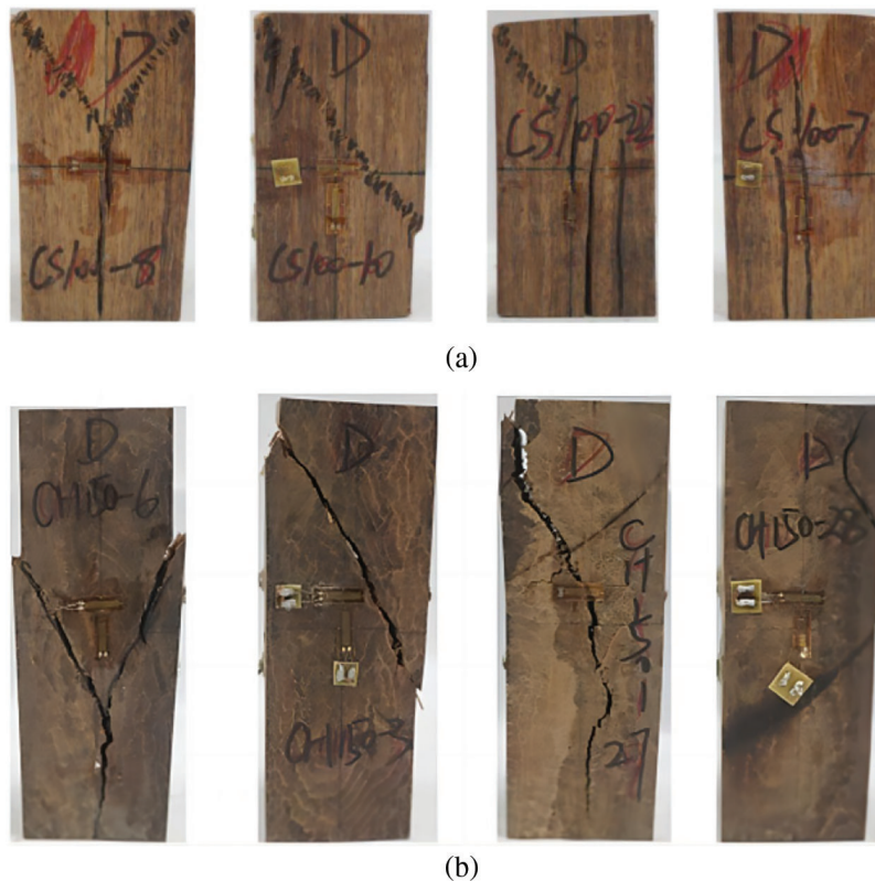
Figure 4: Compression failure forms: (a) parallel to grain. Adapted with permission from [60], Copyright © 2020, Elsevier B. V; (b) perpendicular to grain. Adapted with permission from [69], Copyright © 2019, Tech Science Press
