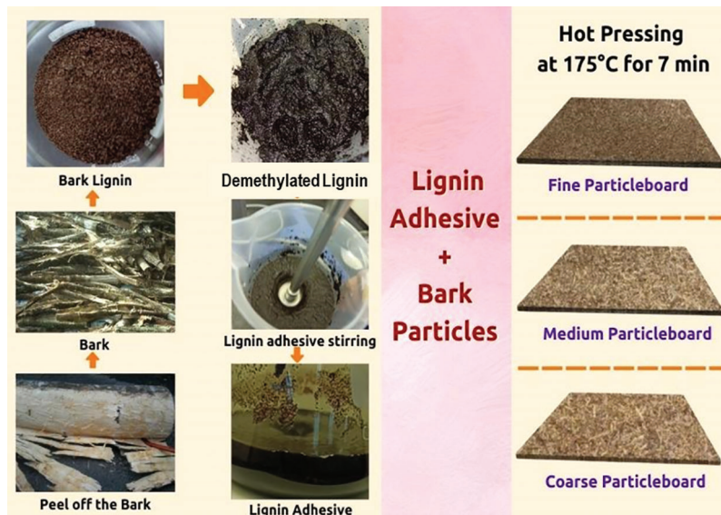
Figure 5: Manufacturing process of bark particleboards with lignin adhesive
