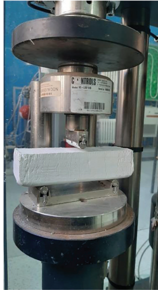
Figure 10: 3-point bending test of plaster-fiber banana y = 0.14
