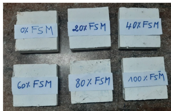
Figure 6: Thermal samples of the composite plaster-fiber banana for different percentages of additives with series model distribution of fiber “FSM”
