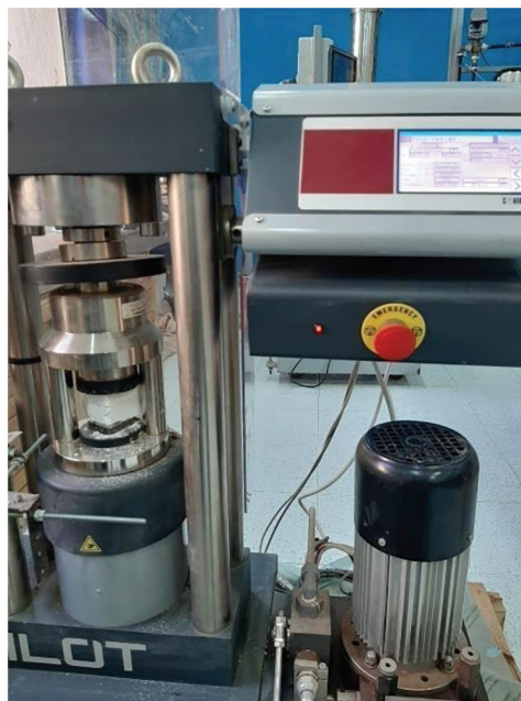
Figure 11: Compression test of plaster-fiber banana y = 0.14
