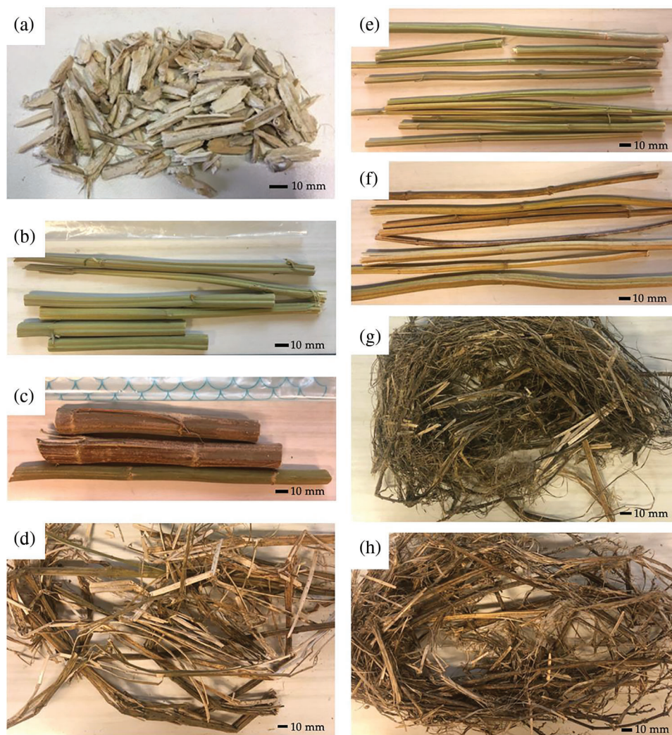
Figure 1: Examined raw hemp hurd. AHMC Frog1: hemp hurd chips (a); CSIRO Frog1: early harvest (b), late harvest (c), baled (d); CSIRO Han NE: early harvest (e), late harvest (f), baled (g), retted (h)
