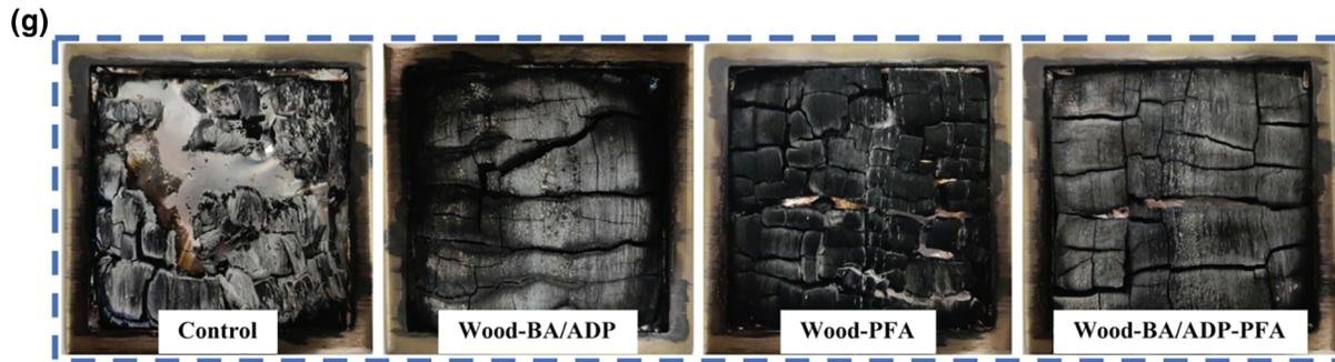
**Figure 5:** The main combustion parameters (a–f) obtained by cone calorimetry of wood and modified wood, along with a photo (g) showing the residual carbon after combustion
