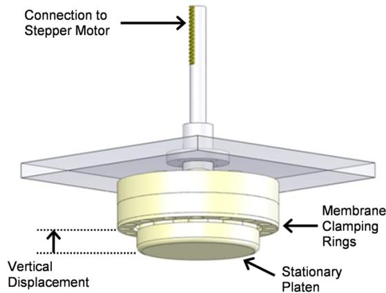
Figure 1: Membrane device schematic: A circular elastomeric membrane was radially deformed by stretching over a stationary platen driven by a computer-controlled stepper motor. Vertically displacing the clamped outer circumference of the membrane produces uniform radial loading of the membrane's edge.
