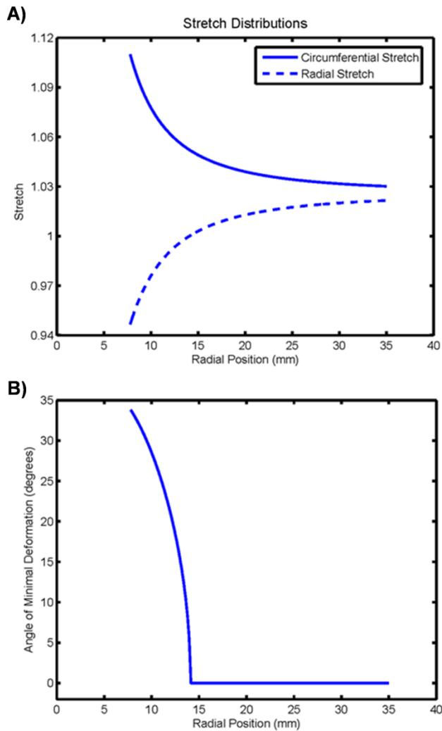
Figure 3: Membrane stretch profile characterization: Radially deforming a circular membrane with a central defect generated gradients in both circumferential and radial stretch components (A). The off-axis direction of minimal stretch varied with radial position due to circumferential: radial stretch ratio variation (B).
