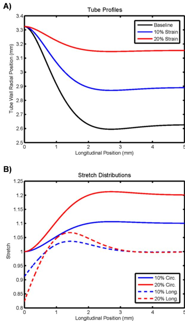
Figure 4: Tube geometries and stretches: A thin-walled tube was implanted with a rigid cylindrical insert and subsequently subjected to cyclic inflation. The tube geometric profile (A) and stretches (B) were calculated for cases of 10% and 20% nominal stretch, defined by the circumferential stretch far from the rigid insert between systolic and diastolic configurations.
