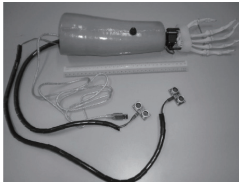
Figure 52: Controlling Prosthesis using Ultra sonic sensor by Razak et al.
