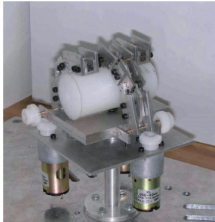
Figure 41: Three-fingered 1-D.O.F LARM hand by Marco Ceccarelli et al.
